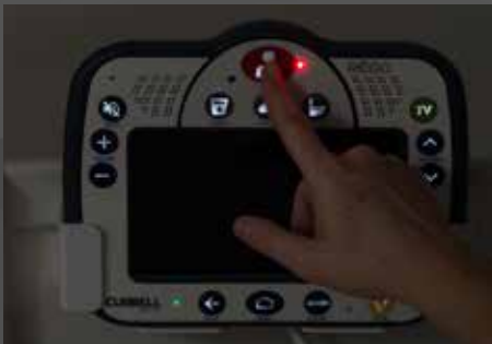
All buttons are back-lit, making them easy to find in the dark. Additional LEDs give visual assurance of various functions.
